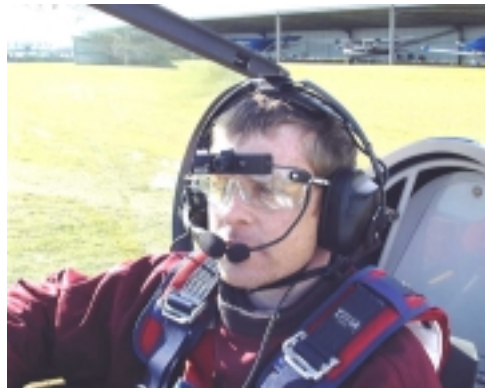
Figure 2-1: The Pilot of an Aerobatic Aircraft Wearing ISECS
