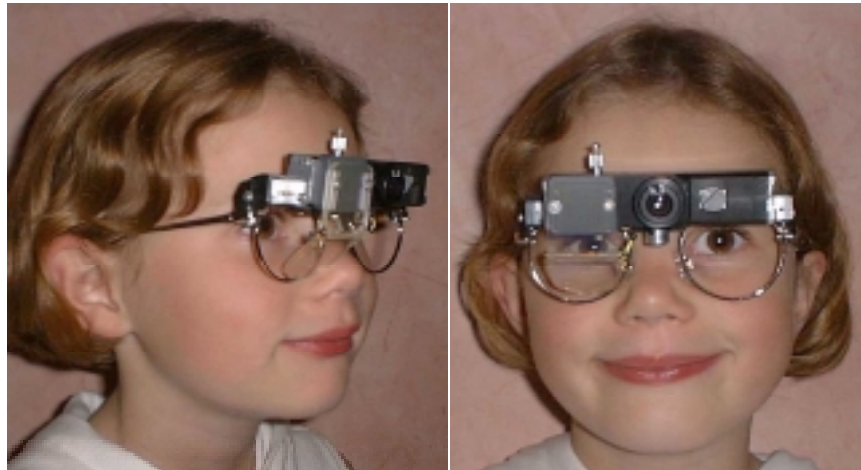
Figure 5-1: The ISECS Module Adapted for Mounting on Children's Wire Frame Spectacles
